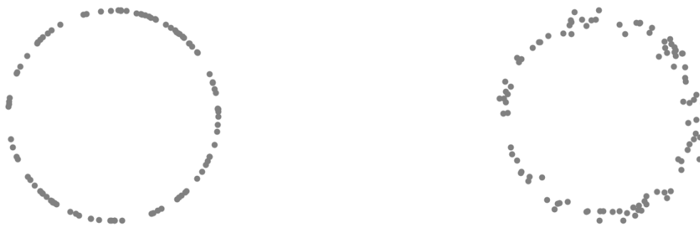
Figure 2.12 Data sampled from a circle with little noise (left) and much noise (right).
